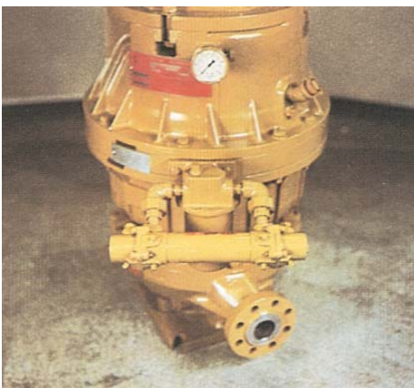
Gearbox Heat Exchanger (Required above 9000 rpm, and/or 350°F process temperature and all full emission models)
