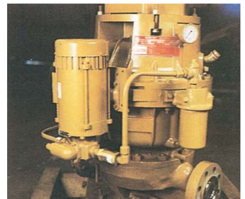
Auxiliary Lube Oil Pump (Required on LMV-331, all full emission units, all horizontal units, or units with gearbox inline heater, air cooled heat exchanger or tilt pad bearings)
